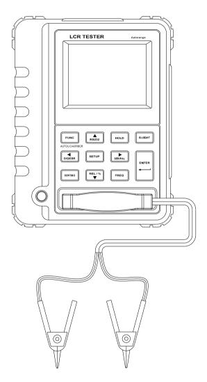
Schematic diagram for using Kelvin clip to measure Remarks: insert the plug correctly according to the diagram. Measurement can't be done if inserted incorrectly.
